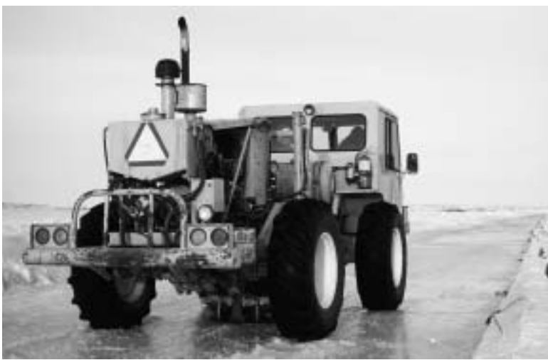
UBC researchers used vibroseis trucks to help them 'map' kimberlite fields in Canada's Northwest Territories.
