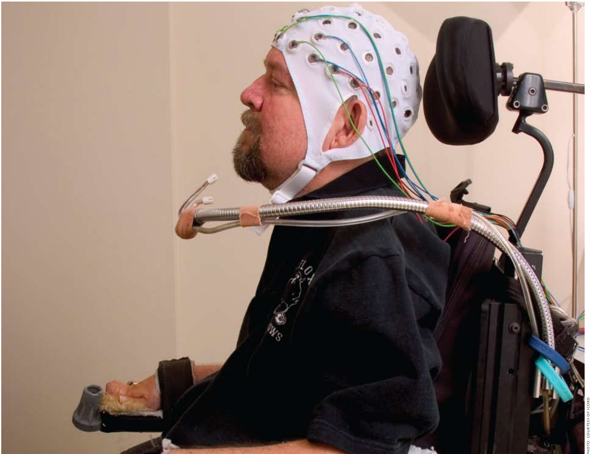
Tetraplegic Don Danbrook demonstrates a prototype BCI recording cap.
